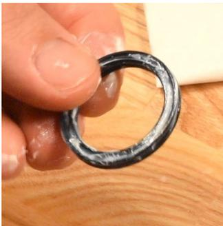
Apply only a thin film of P10L grease to the X-ring seal to aid in installation.
