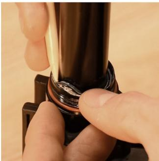
When installing the X-ring into the Collar Nut, be careful to work it in gradually using a blunt tool. It must be fully seated into the Collar Nut, or else the SSR will be over compressed when the Collar Nut is tightened and the benefits of the SSR will be diminished or lost.
